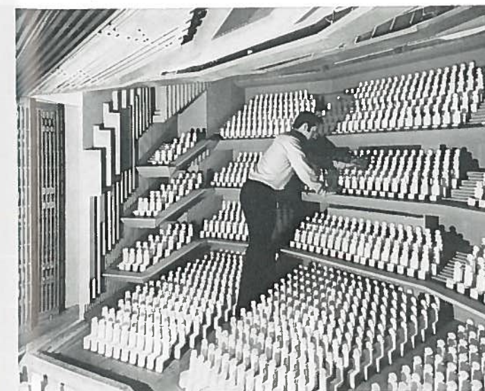
Eighth-scale model of the auditorium for acoustic and climatic tests. (The detail of the wall treatments is provisional and merely stands for something which will be there but has yet to be designed.)
