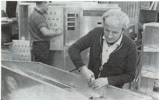
The metal work for dimmer racks and control desks is fabricated ...
