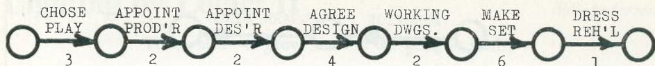
Fig. 3. The diagram shows the sequence and duration of activities necessary before the scenery can be ready for the First Night. Minimum time—20 weeks.
