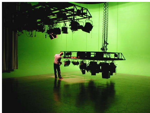
A technician works with Quartzcolor luminaires on one of the motorized grid sections.
