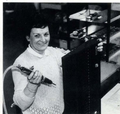
Irene Dryburgh using a compressed air screwdriver on Action final assembly.
