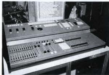
2. A Task Master desk-top section of console, above a Lightboard M1 — can control any number of lights on 99 channels with 250 memories. Left of centre is the track ball for pan & tilt setting.
