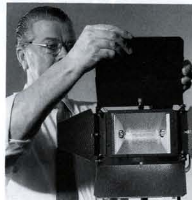
2. Sliding in the barndoor reflectors. These can act as a beam intensifier if the reflected light is directed into the centre of the beam, producing double the light level. Or, directed to the outside of the lit area, they increase the beam angle.
