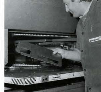
3) A component emerges from a programmed turret head punch.
