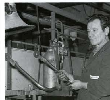
5) Welding up the yoke.
