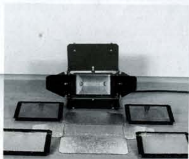
5. Here is the Iadi Fill, which has a unique reflector profile providing a wide angle even fill beam ideal for lighting large areas in places where height and distance are even more restricted than usual. Also shown are the specular aluminium reflectors which clip inside the integral barndoors, two alternative wire scrims of different gauge, an opal glass to soften the light and a dichroic coated glass filter to correct 3200°k to match daylight.
