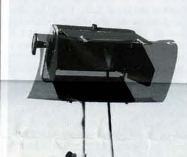
4. The barndoors have clips on their outer edges which hold colour filters a good distance from the lamp and with all the ventilation any filter could desire.
