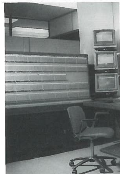
The Mchat Theatre Moscow Galaxy set up for final testing at Brentford before packing. Note the 320 channel four pre-set manual desk for visiting companies not used to memory system operation. Over a kilometre of control cable will be needed in the control room.
