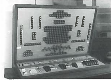
The geographic push button mimic and the stalls control.
