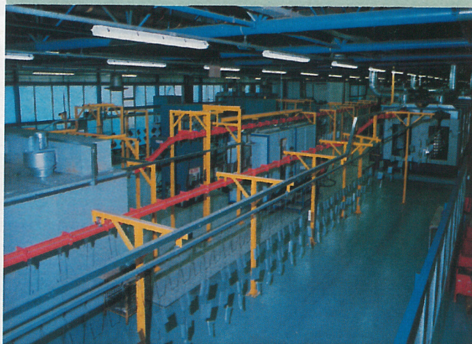
(Left) Automatic preparation and electrostatic powdercoat paint spray process plant. Occupies approximately 5000 sq.ft.
