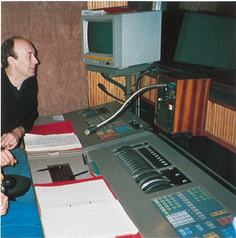
The Siemens B40 control desk at the Royal Opera House.
