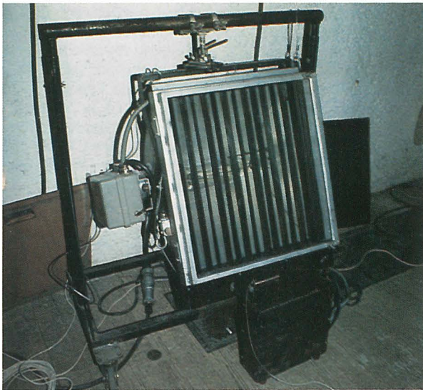
A favourite unit of Max Keller's at the Kammerspiel is this 3500 watt mercury vapor instrument, shown here with a mechanical douser for dimming.
