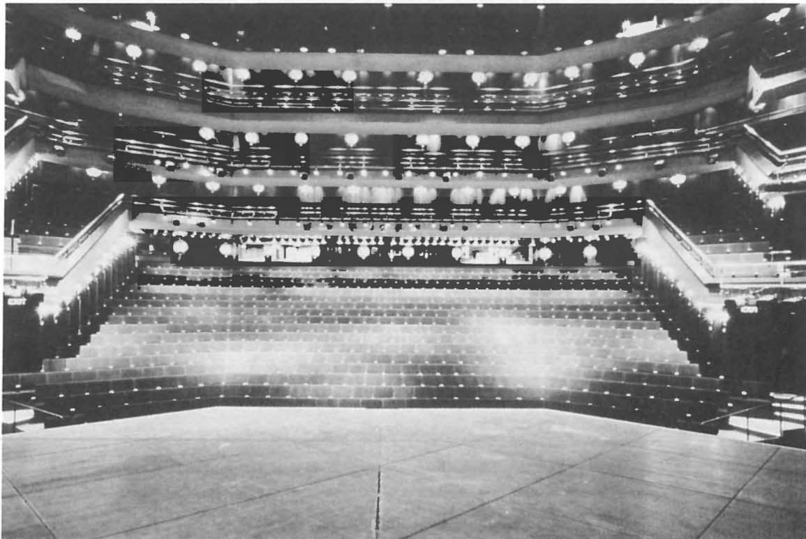
Looking out to the auditorium with the three circles and lighting bridge above from a centre-stage position, approximately 7 metres from the front edge of the stage. The back wall and control rooms behind seem deceptively close. The 'papering' the walls with people with the three side circles also adds greatly to a general feeling of intimacy.
