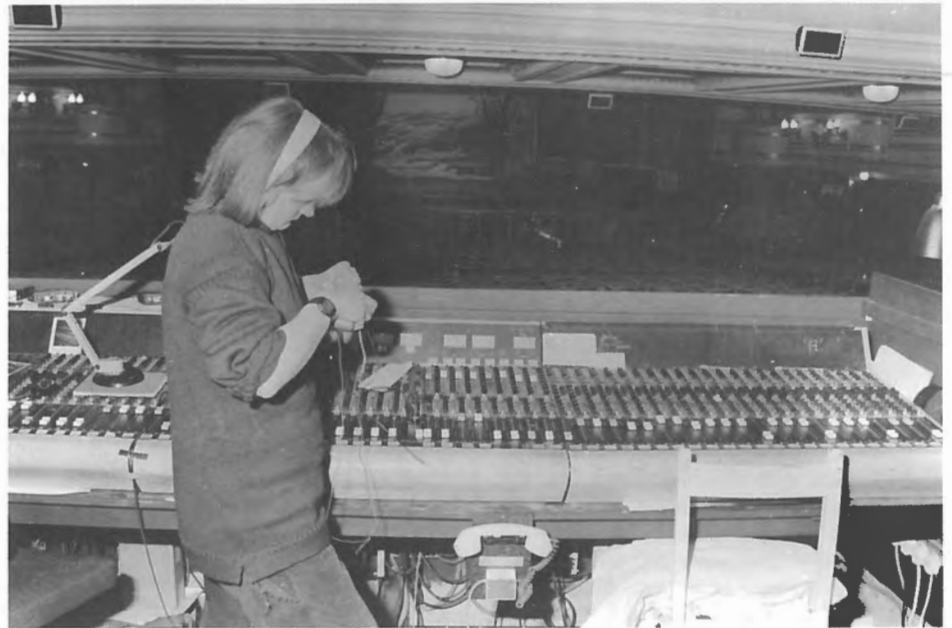
Good performance from the radios is ensured by a lengthy and painstaking setup routine for each performance and rehearsal. The channels are checked visually and for performance — cables, connectors and capsules, and batteries are checked for short-circuit current before they are allowed into a transmitter. In this photograph, four of the under-balcony loudspeakers can be seen, one partly obscured by the operator's head. No justice is here done to the scenery, but the operator's remoteness from the sound of the performance is suggested not too misleadingly.
