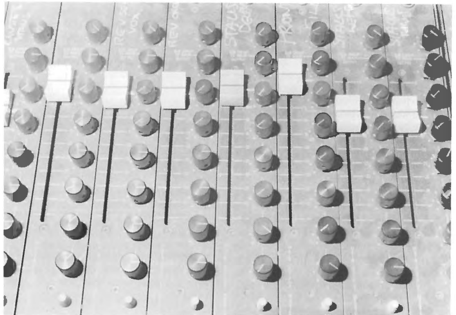
The master output faders of the Trident desk with the operators labelling just legible. The eight level controls alongside each fader control the level of eight subgroups into the master output. The faders for these subgroups are immediately below the master faders and, perhaps confusingly, directly in line with them.
