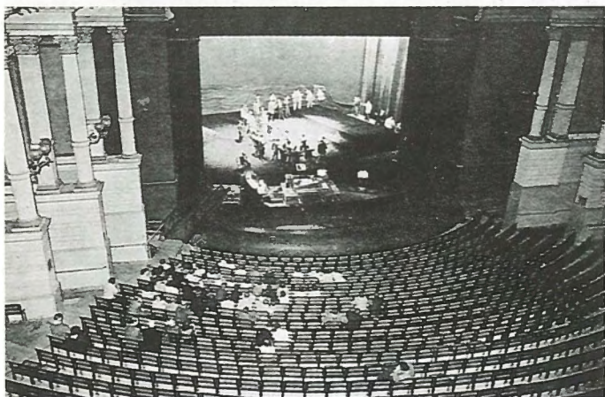
Festspielhaus, Bayreuth – 1876 – auditorium and stage; Putting a roof on an amphitheatre is the most dangerous acoustic practice. Cremer describes the insistence by King Ludwig II that the rear wall be covered with boxes above the amphitheatre for the high society, and above these for their attendants as acoustic luck.
