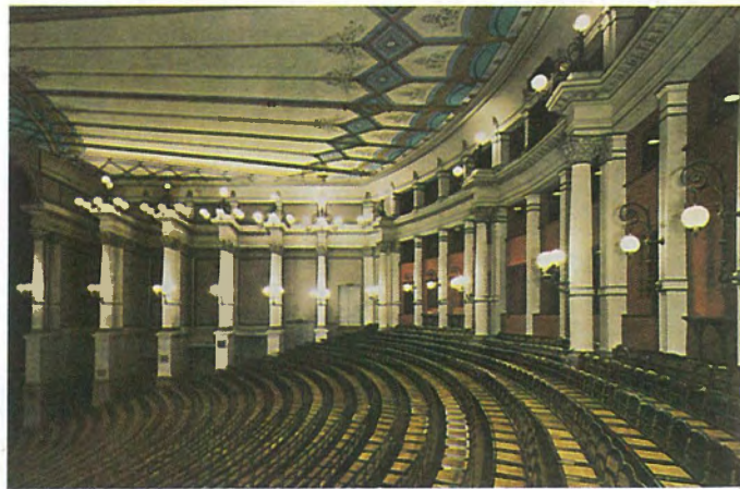
Festspielhaus, Bayreuth – 1876 – auditorium and stage; Putting a roof on an amphitheatre is the most dangerous acoustic practice. Cremer describes the insistence by King Ludwig II that the rear wall be covered with boxes above the amphitheatre for the high society, and above these for their attendants as acoustic luck.
