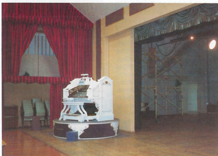
The Wurlitzer Organ is mounted on a turntable which travels on an elevator in the stage apron.
