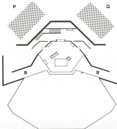
This diagram indicates a conventional 'box-frame' drawing-room set on the open stage. In this instance the stage ramps B are not normally used. Actors' entrances are through the doors and arch of the set upstage.
