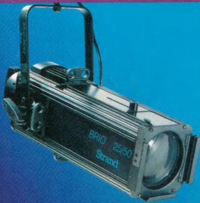
The restyled Brio 18/30 and 25/50 600W Zoom 'Coolbeam' Profile Spotlights are high-efficiency, glass dichroic reflector spots, designed for superb performance and based around the HX600 lamp. This means that the front of the lantern and gate area remain cool.
