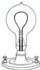
THE first incandescent electric lamp was invented by Edison in 1879 and was provided with a filament made by the carbonization of a bamboo fibre.
