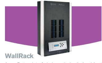
A cost effective solution for both centralised or distributed dimming installations. Twenty-four 10A dimmers or six 25A dimmers, high performance thermal magnetic circuit breakers prevent nuisance tripping, dual DMX inputs, analogue output, panic or work light preset. Convection cooled, no fans yet compact.
