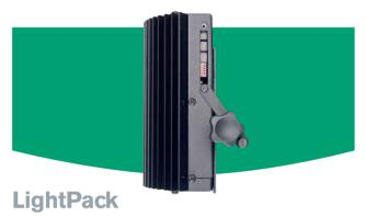
Single I200W IGBT dimmer pack delivering all the advantages of IGBT control — silent, high performance (650uS rise time, insertion loss of I.5V), able to precisely control LED, transformer as well as tungsten halogen loads.
