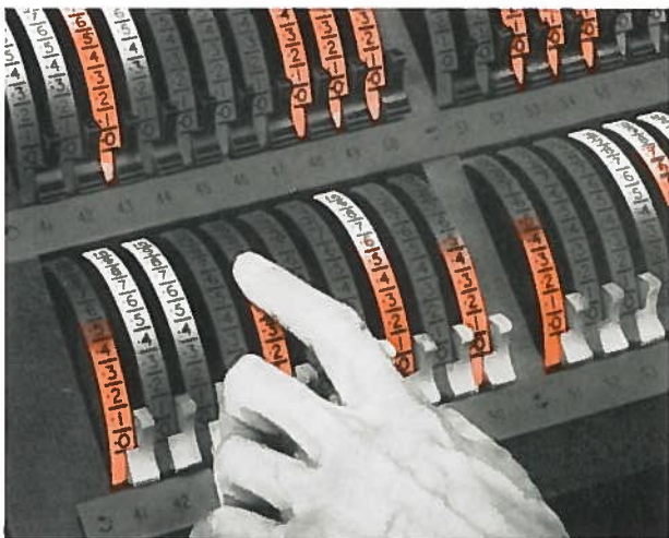
The luminous dimmer lever exclusive to Rank Strand control systems.
