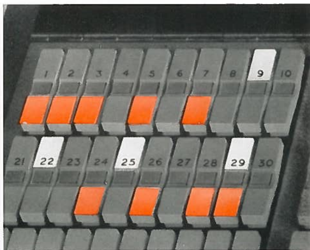
The illuminated rocker dimmer switches designed for Rank Strand memory controls.
