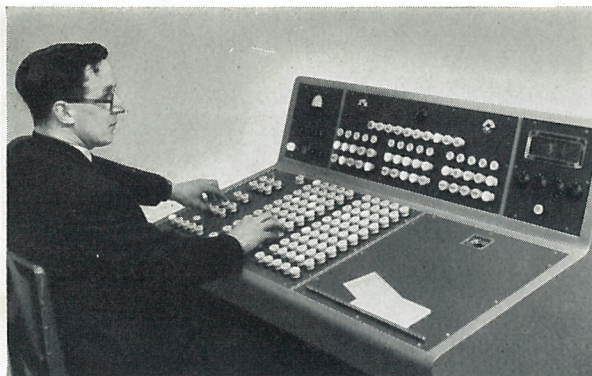
Strand system KTV, (patented). The first dimmer system with fully automatic plotting of lighting and switch-board controls in the world (April, 1959).
