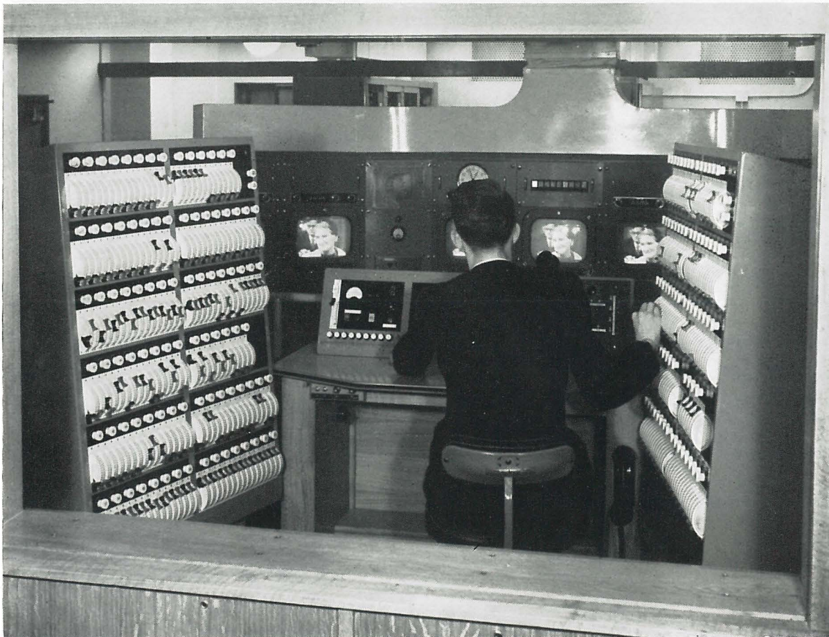
The Strand system C Console-Preset control installed in the British Broadcasting Corporation's Television Studio 'Riverside I'.
