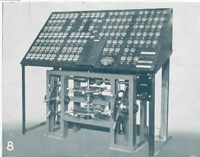
Covent Garden Opera House Dimmer Control
