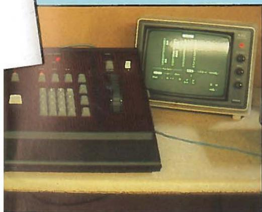
stored two different tones, one 800Hz signal and one 1.5kHz signal. When the 800Hz signal was played back to a special device it would close a relay and the relay closed the external fade function on the M24. At every place in the show where we wanted a change in the light we recorded an 800Hz signal on our audio channel. The 1.5kHz signal closed the No. 1 button on the keyboard.
