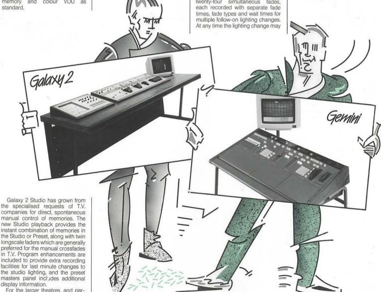
the specialised requests of T.V. companies for direct, spontaneous manual control of memories. The new Studio playback provides the instant combination of memories in the Studio or Preset, along with twin longscale faders which are generally preferred for the manual crossfades in T.V. Program enhancements are included to provide extra recording facilities for last minute changes to the studio lighting, and the preset masters panel includes additional
