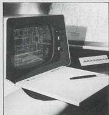
We use the light pencil method of P.C.B. design.
