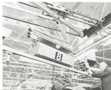
A self climbing hoist fixed to a beam, which can pivot and traverse, undergoing factory tests.
