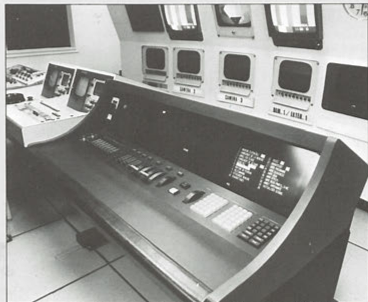
Strand Light Palette Memory System, with French language on the V.D.U.'s.
