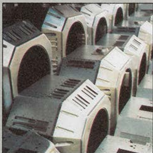
A close-up of newly-formed housings prior to painting and final mechanical and electrical assembly. Once complete, these will become "Kahouteck" dual-purpose spot/softlights. (Photo by Randall Miles ARPS, AFIAP, MBKS)
