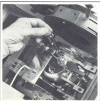
Reflector and condenser system of the Niethammer followspot. Get that rigid construction! Note the interlock safety switch.
