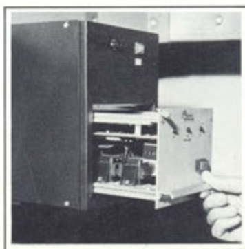
▲ Rank Strand Load Limiter as installed at Wyndhams Theatre. There is a control which sets the load at which the device automatically comes into action, and the fault corrected or the stage lighting varied as compensation by use of the M.M.S. auto mod facility.
