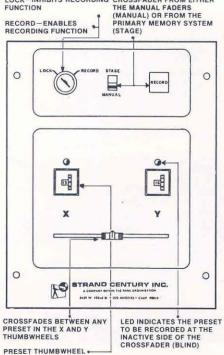
window. The system is self-contained within its desk which includes twin powerpacks. The edge of the desk is padded to provide a comfortable rest for the operator's forearms and wrists.
