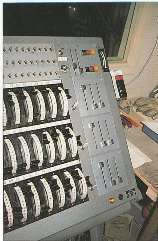
JP control modified to allow formation of 3 separate groups within each of the three Presets, with optional selection to Crossfader—Unge Nye Theatre, Oslo.
