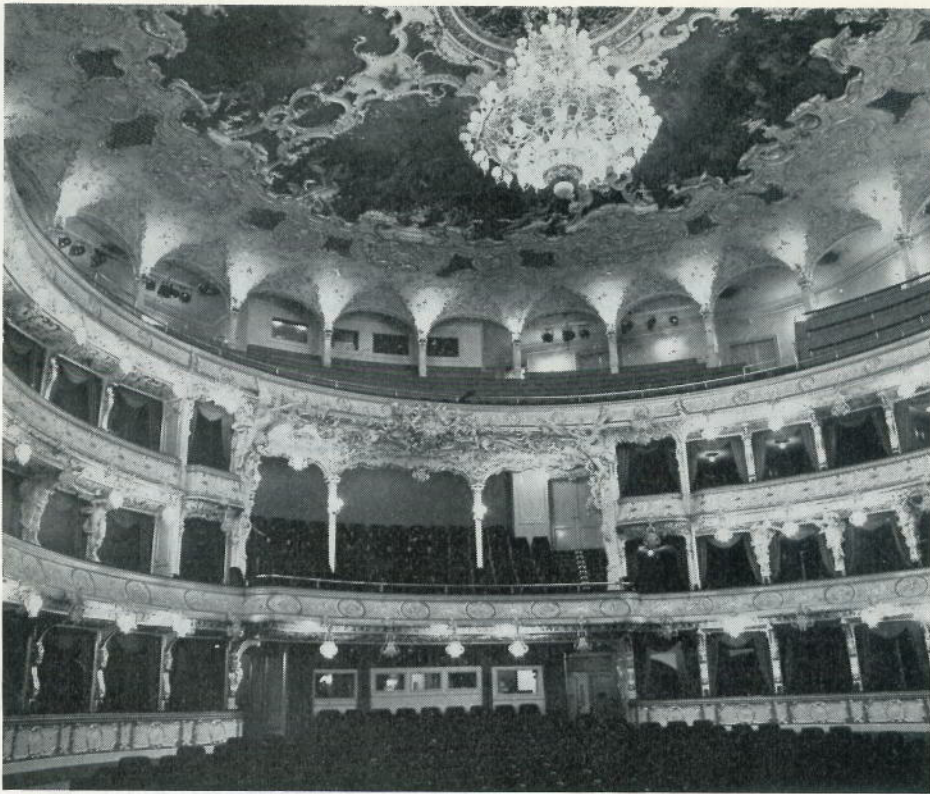
Smetana Theatre, Prague. Note lighting positions in roof arches. The Control Room is seen at back of stalls.
