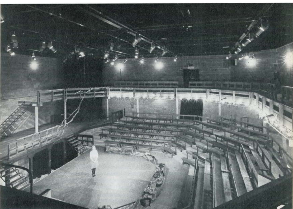
Young Vic Theatre. Lighting grid, access only from below by Tallescope. Thrust stage in low position.
