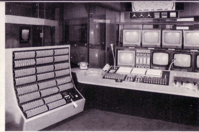
Lighting control and mimic diagram, BBC T/V Centre, Studio 6.
