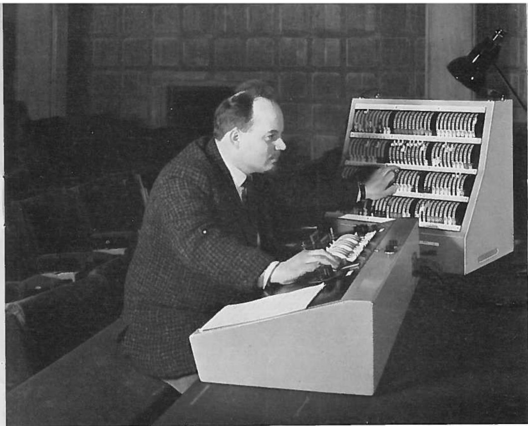
Fig. 1. Francis Reid at the portable control position in the stalls. 120 dimmer channels on his left and full set of master controls on his right.
