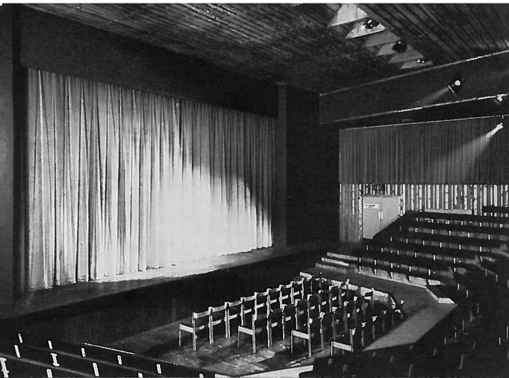
Fig. 1. Goldsmiths' College Theatre. As proscenium stage with forestage lowered and temporary stalls seating partly in position.
