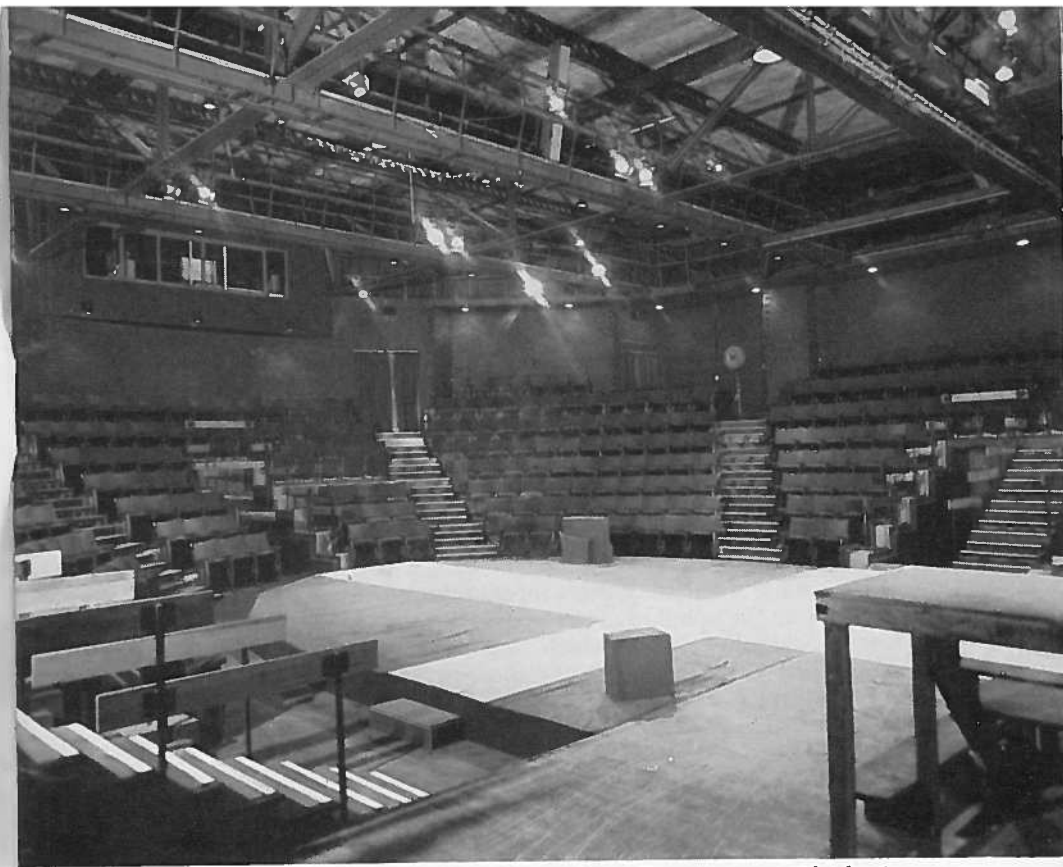
Fig. 1. The Questors Theatre, Ealing. View from off-stage prompt side showing lighting bridges overhead and control room top left.
