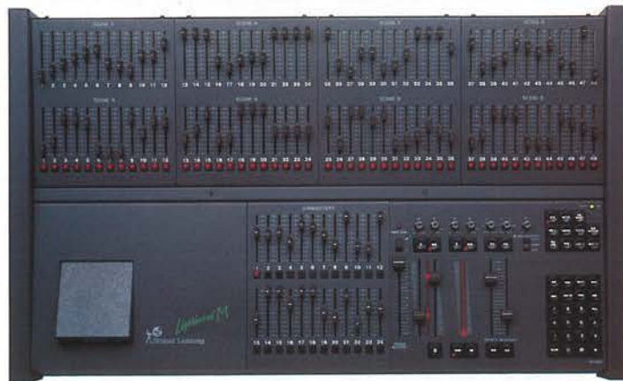
Lightboard M - A 96 channel Memory with Manual System
