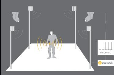
Local position measurement Performers are equipped with a transponder. The position is calculated to within +/- 2 inches accuracy.
