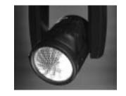
The VARI\*LITE® VL5Arc™ wash luminaire uses a 575W, 5600°K arc lamp, combined with the VARI\*BEAM™ mechanism. This diffusion device uses a fluid-filled plastic membrane to provide powerful automated beam angle variation.
