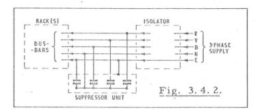
Note that the common terminal of the Suppressor Unit capacitors is taken to the Neutral line. Local electricity-authority regulations may require the Suppressor Unit to be separately fused on each phase.
