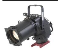
A base down axial ellipsoidal delivering a "cool" beam of light in a beam range adjustable between 45° to 75°. The beam is crisp "white" light with little or no distortion in the range of 45°-65°, ideal for gobo projection and precise beam shaping.
