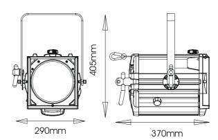
Weight: Packed Weight: Colour Frame Size: Included: 5.3kg 6.2kg 186mm x 190mm 1 x colour frame, yoke nut & bolt, instruction leaflet.
