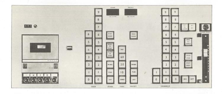
For ease of operation, the controls have been arranged in two basic groupings representing those required for rehearsal and those for an actual show. All push-buttons illuminate when depressed, the preset functions showing as blue for ease of identification.
