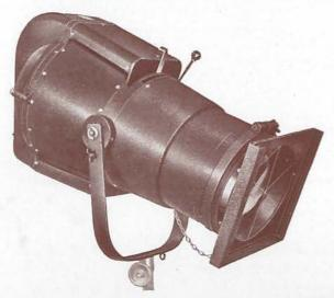
This lantern gives a high power, narrow angle clear cut beam of twice to three times the intensity of the standard Mirror spot. Beam shape and size is adjustable by iris diaphragm and foursided masking shutter.
