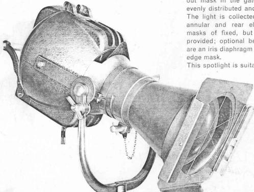
This spotlight projects a high intensity narrow angle beam of any profile determined by a cutout mask in the gate runners. The beam is evenly distributed and has clear cut edges. The light is collected at the gate by a front annular and rear ellipsoidal reflector. Four masks of fixed, but different, apertures are provided; optional beam-shaping accessories are an iris diaphragm or an adjustable straight-
