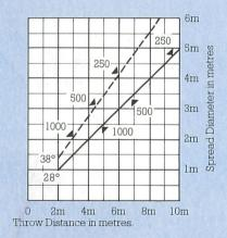
The figures on the diagonal lines indicate the illumination value in lux at beam centre.
