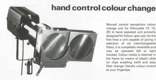
Manual control semaphore colour change unit for Silhouette 10, 15, 25. A hand operated unit primarily designed for follow-spot use; for the first time a unit capable of giving a selection of six interchangeable filters, it is completely reversible and may be operated left or right handed. Colour media is retained in the frame by means of plastic slide on clips enabling swift and easy filter change; literally colour control at your fingertips.
