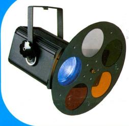
Remote control 24V AC Chromatic Wheel system with five colours and continuous selection. Standard controls for up to ten units in any combination of two, four or six groups operating on ring of three 0.5mm² control cables. ColorPad Matrix with status feedback. Wheel and Semaphore systems are available for other CCT luminaires.
