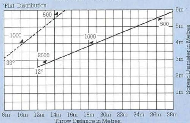
The figures on the diagonal lines indicate the illumination values in lux at beam centre.
