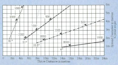
The figures on the diagonal lines indicate the illumination value in lux at beam centre
