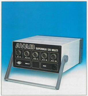
The AVAB demultiplexer converts the digital multiplex signals from the 202 into analog control voltages. AVAB makes demultiplexers for every application: for permanent installations, where the unit can be placed in close proximity to the dimmers, or for portable use, where it is completely self-contained with all necessary input/output ports. The control voltage can be adjusted internally to interface with most analog dimmers on the market.
