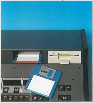
The external memory of the 202 is the new standard 3.5-inch floppy disk drive. Not only does the floppy disk drive provide library storage for all your lighting programs, but also extends the usable memory of the 202 during performance. A read-from-disk command, namely, accesses information on the diskette automatically as it is needed, thereby increasing the capacity of the 202 to provide as much memory as is required.
